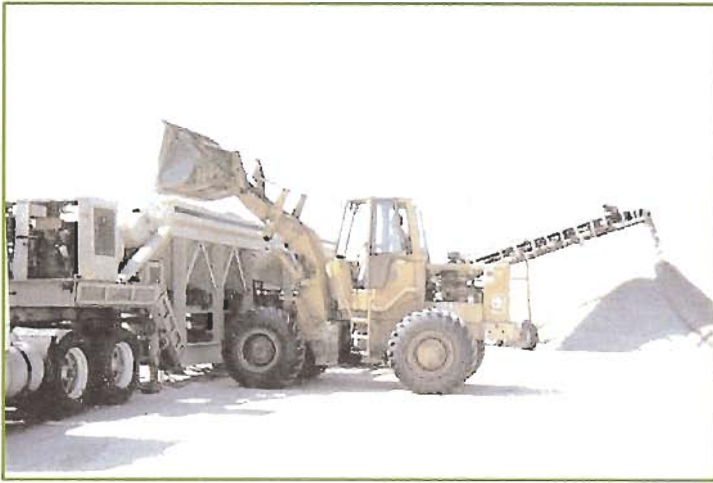
Figure 6 – Rootzone components must be blended uniformly. Mechanical blenders are best suited to this task.
